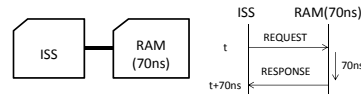
図4 SystemC TLMにおけるプロセッサと外部モデルの通信 Fig. 4 Communication between a processor and external model in SystemC TLM
