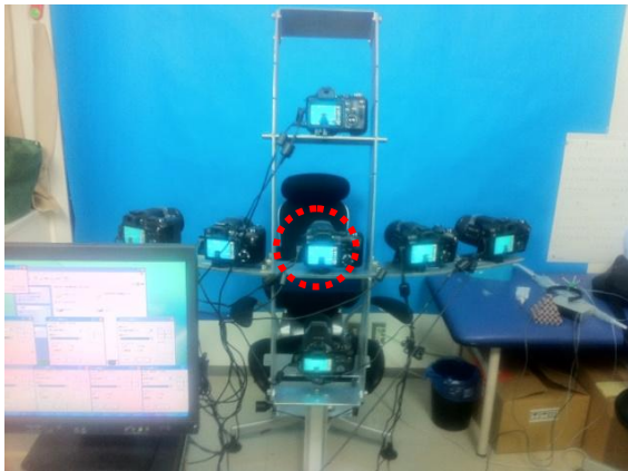
図 6: Synchronous Multi-Angle High-speed Capture System : SMAHCS
