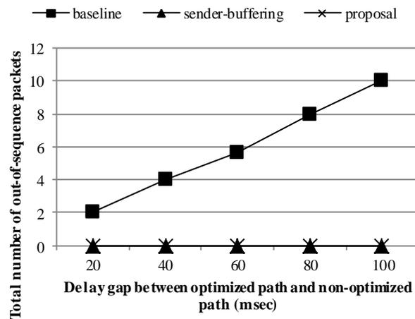
Fig. 7 Number of out-of-sequence packets vs. delay gap between optimized path and non-optimized path ( $d_l = 50$  msec).
