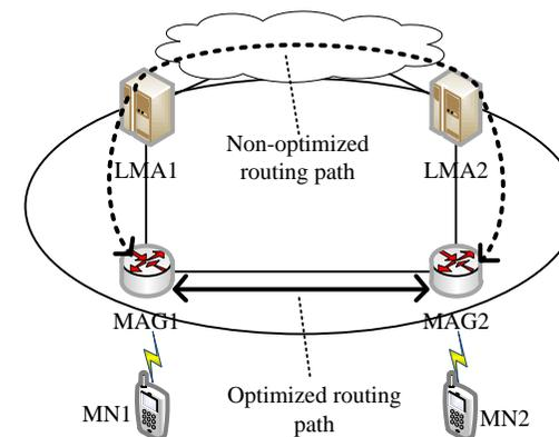
Fig. 1 PMIPv6 domain with non-optimized and optimized routing paths
