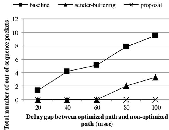
Fig. 6 Number of out-of-sequence packets vs. delay gap between optimized path and non-optimized path ( $d_l = 30$  msec).
