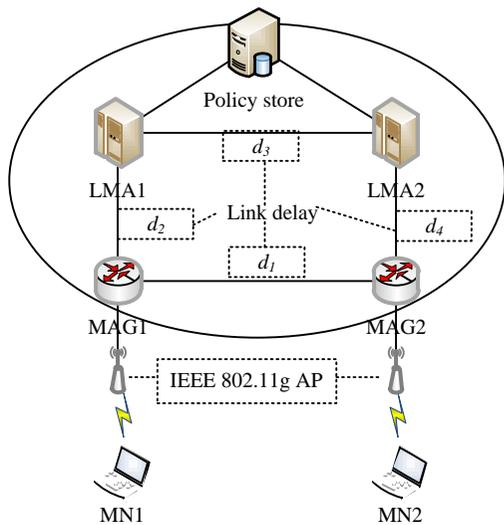
Fig. 4 Network topology of experimental testbed.
