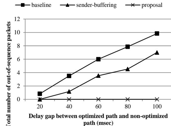
Fig. 5 Number of out-of-sequence packets vs. delay gap between optimized path and non-optimized path ( $d_1 = 10$  msec).
