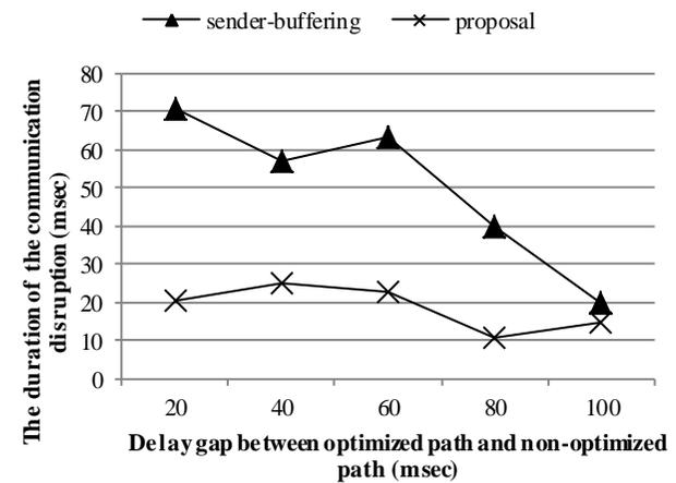
Fig. 8 Duration of communication disruption during route optimization ( $d_l = 50$  msec).
