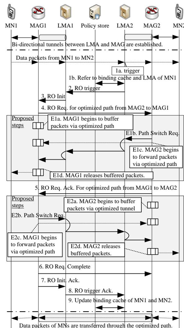
Fig. 3 Route optimization procedure with optimized path switching. Signaling messages are indicated by a solid line while data packets are indicated by a dotted line. The procedure regarding the optimized path switching is enclosed by boxes.
