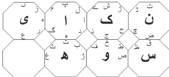
Figure 3 Proposed keypad for touch screen mobile phone.
