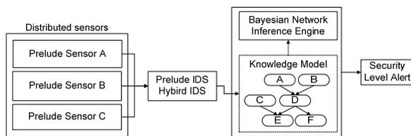
Fig. 2 System architecture
