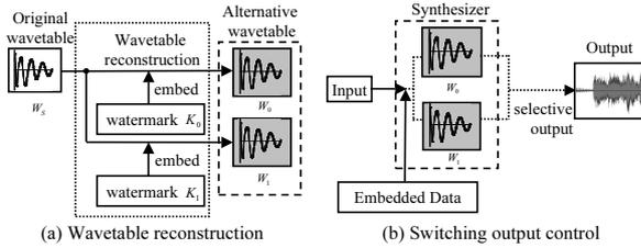
Figure 1: Systematic flow of the proposed scheme
