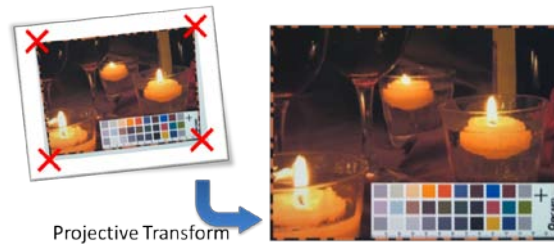
図 3 射影変換例 Figure 3 Example of projective transform.
