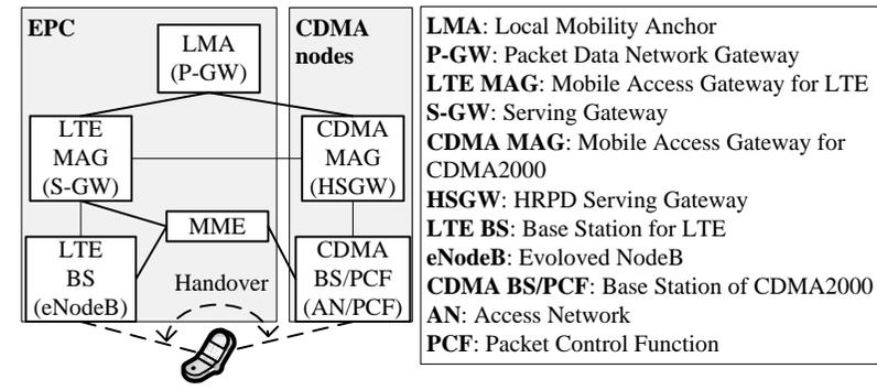
Fig. 1 SAE architecture including CDMA2000 nodes.
