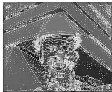
図 7 特徴点の動き推定結果 (5,333 点) Fig. 7 Feature points and estimated motions(5,333 points).
