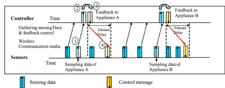
Figure2. Packet delivery in sensing and feedback control
