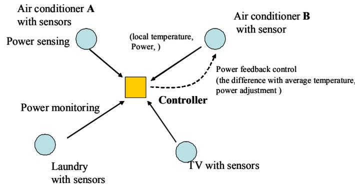
Figure1. An example of sensing-control model
