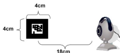
Fig. 4 Experiment setting used of which the webcam is located at 18cm from the 2D marker
