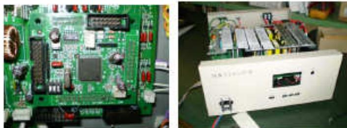
Fig.7 Actual Inverter Power Supply Device
