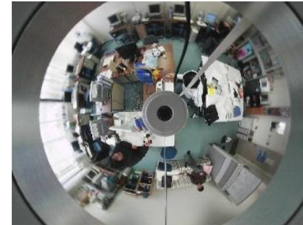
Fig.2 An image taken by omni-directional camera.
