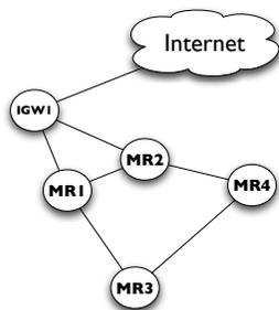
Fig. 3 Example of topology in MANET.
