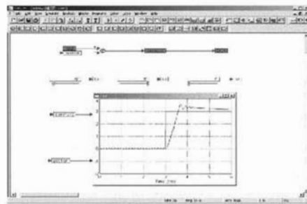
Figure 12. The PID control experiment K_p=48 K_i=0.05
