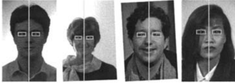
Fig. 9 Results of the facial feature extraction where the midlines are employed as guide for restriction to the vertical scan-line number of one.
