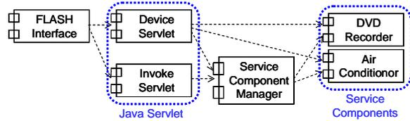
Fig. 4: Structure of SOA-based HNS
