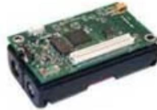
Figure 6 : MicaZ mote sensor node
