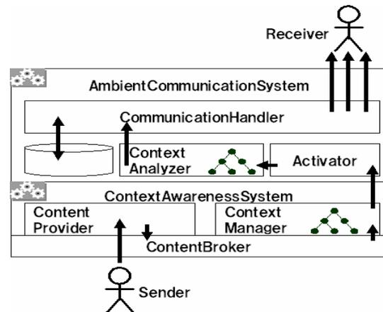
Fig. 7 Schematic View of Architecture
