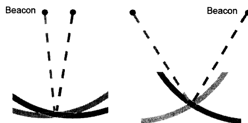
Figure 3: On the left is an example of close alignment of beacons. On the right is a wide alignment of beacons.
