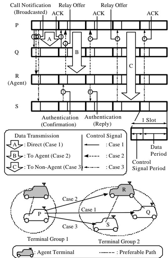
Figure 4: Time-space diagram of proposed algorithm.
