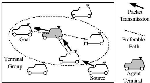
Figure 1: Concept of packet routing.
