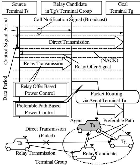
Figure 5: Transmission power control for proposed algorithm.
