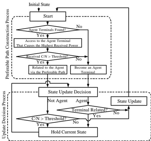
Figure 2: Flow Chart for Terminal Group Construction.
