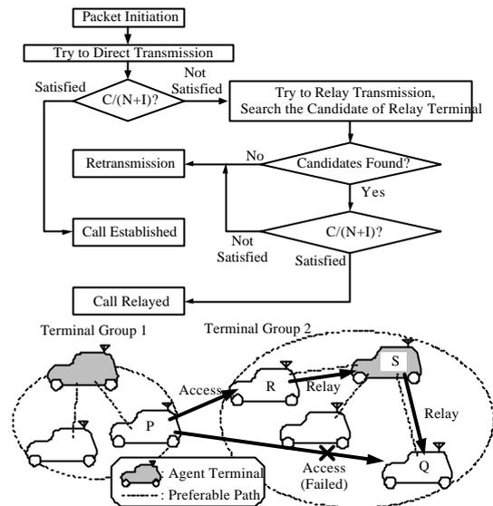
Figure 3: Packet routing scheme.
