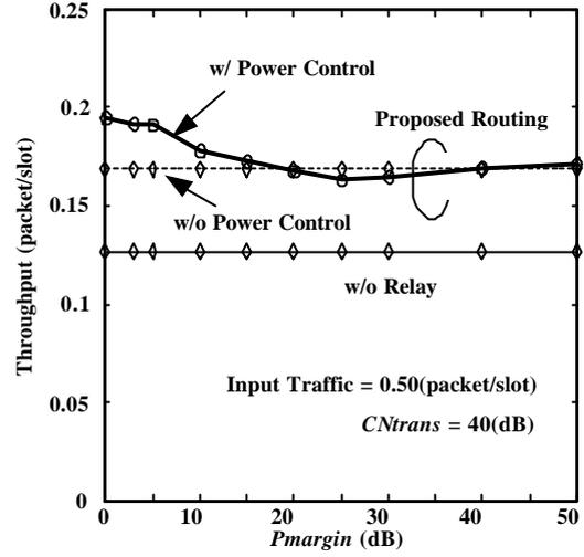
Figure 8: Throughput versus  $P_{margin}$ .
