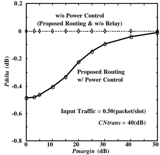
Figure 9: Average transmission power versus  $P_{margin}$ .
