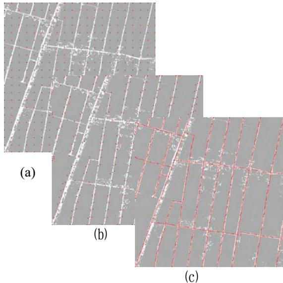
**Fig. 9** The Results of SOM and Road Tracked Process for the Large Field Road Image (a) 50 Pixels Initialization Grid (b) After twice iterations (c) Road Network Extraction
