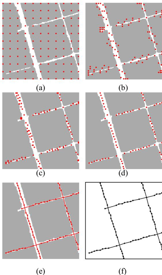
**Fig. 5** The Process Results for the Small Field Road Image (30 Pixels Initialization Grid) (a) 30 Pixels Initialization Grid (b) After twice iterations (c) After 4 time iterations (d) After 10 time iterations (e) Road Tracked Linking (f) Road Network Extraction
