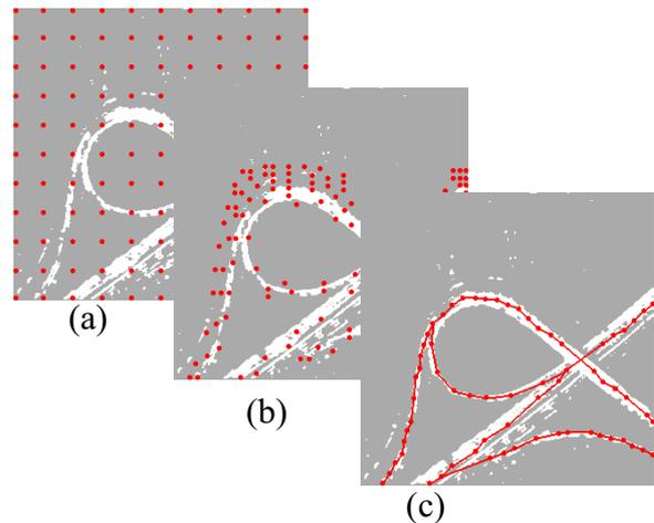
**Fig. 6** The Process Results for the Small Overpass Road Image (30 Pixels Initialization Grid) (a) 30 Pixels Initialization Grid (b) After twice iterations (c) Road Network Extraction
