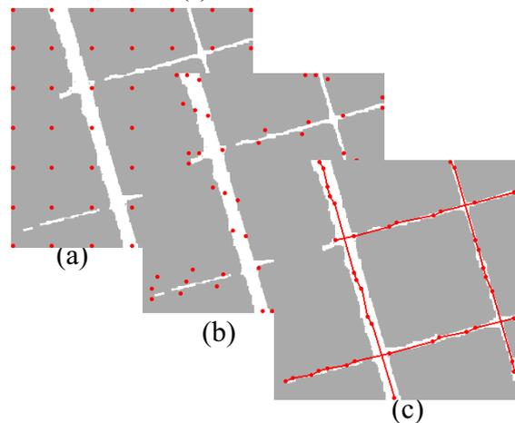
**Fig. 7** The Process Results for the Small Field Road Image (50 Pixels Initialization Grid) (a) 50 Pixels Initialization Grid (b) After twice iterations (c) Road Network Extraction
