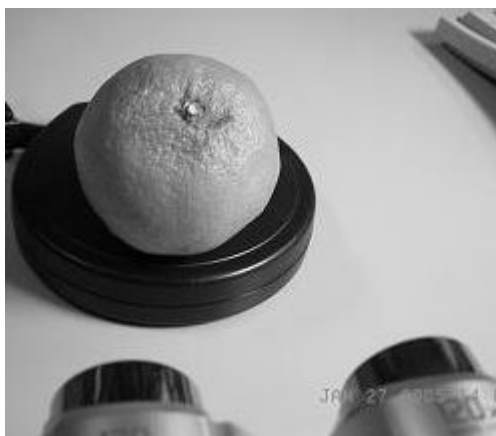
Fig. 3. Mandarin Orange placed for remote stereo observation, with the pair of stereo cameras pointing to the objective
