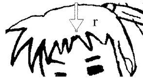
Figure 2: Centroid of a region r . For example, if r is the hair region, its centroid is at the tip of the arrow.
