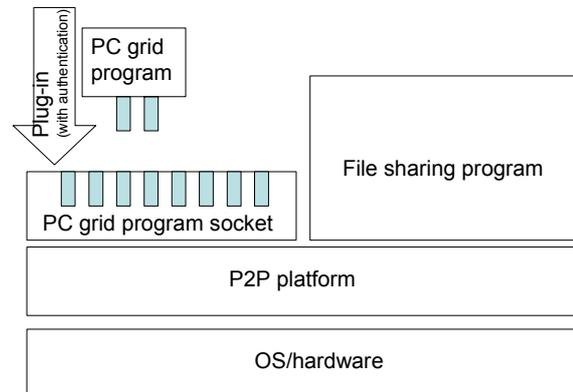
**Figure 3. Software implementation of YOHEIX in a user's PC (peer).**
