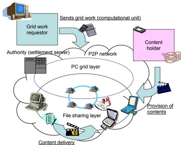
**Figure 2. PC grid-file sharing hybrid system: YOHEIX.**
