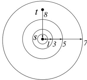
⊠ 1: Illustration of the doubling algorithm. Numbers represent transmission times, with the transmission range doubled by the sender  $s$  at each round until reaching the receiver  $t$ .
