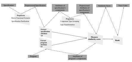
Figure 5. Workflow of establishing SOFL-to-Java trace links.
