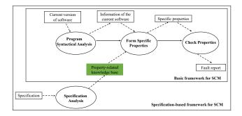
Figure 1. Specification-based framework for software construction monitoring.
