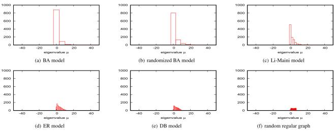
Fig. 4 Histogram of eigenvalues  $\mu$  of a Laplacian matrix for a network instance (N = 1,000 and  $\overline{k} = 4$ ).
