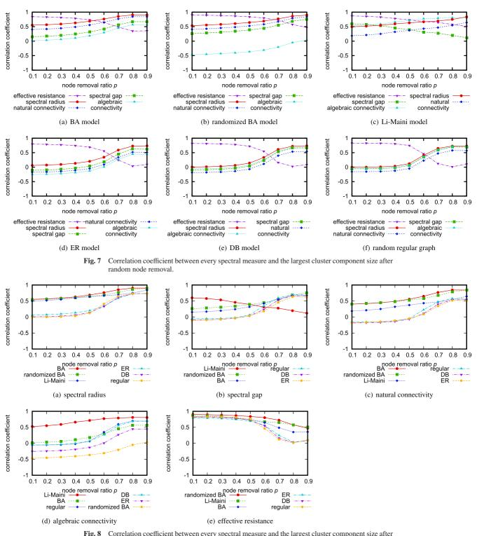
**5.8** Correlation coefficient between every spectral measure and the largest cluster component size after random node removal for different network generation models.
