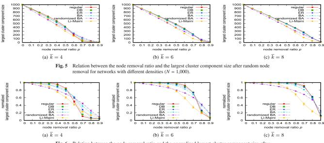
Fig. 6 Relation between the node removal ratio and the normalized largest cluster component size after random node removal for networks with different densities (N = 1,000).
