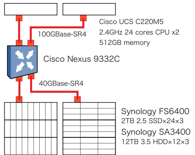
**Fig. 1** A diagram of benchmark setup for IOzone
