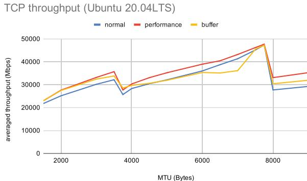
**Fig. 2** TCP throughput changes and MTU change on Ubuntu 20.04 LTS
