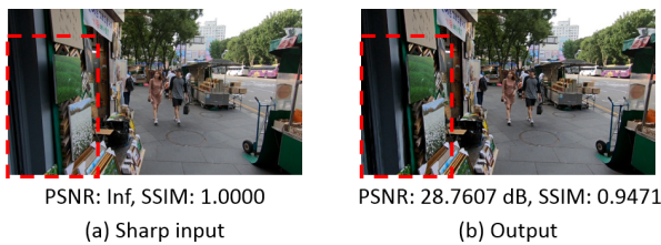
Fig. 3 Illustration that EDVR seriously worsens the sharp input since it cannot discriminate the sharp information.
