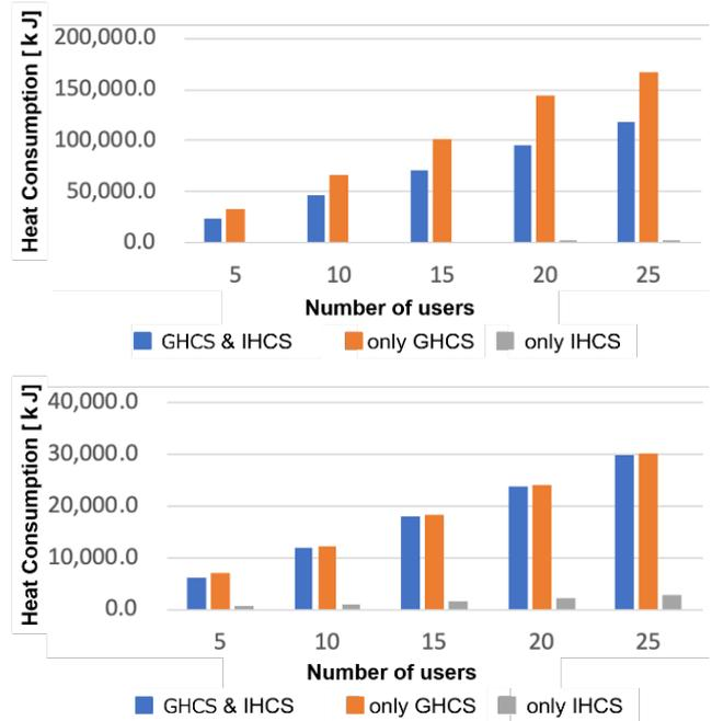
Fig. 3 Total heat consumption in cooling (top) and heating (bottom) conditions of each system depending on the number of users in the room
