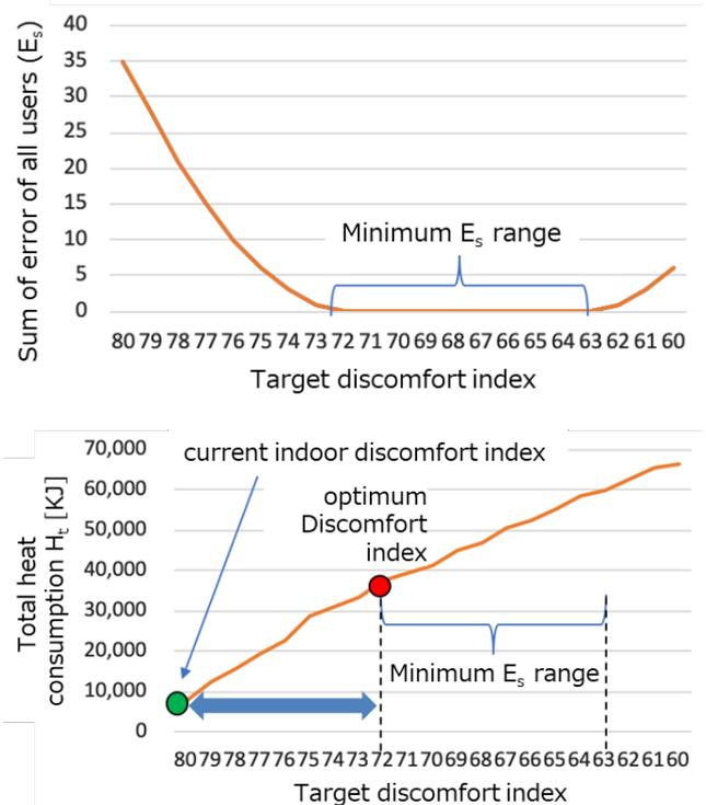
Fig. 2 Method to detect the optimum target discomfort index from the change of  $E_s$  (top) and TDI (bottom) regarding environment discomfort index
