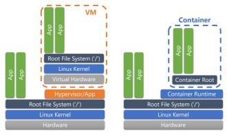
Fig. 1 Overview of virtualization technologies: hypervisor-based (left) and container-based virtualization (right)
