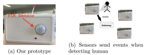
Fig. 1 PIR Sensor (Binary Sensor).
