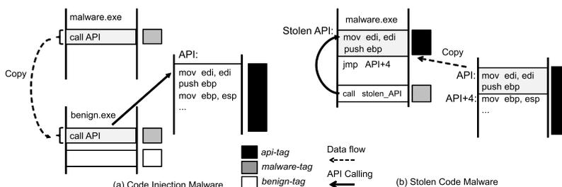
Fig. 3 Taint-based control transfer interception against anti-analysis.
