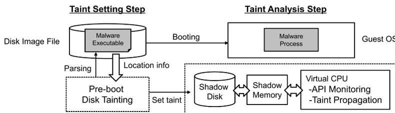
Fig. 4 Analysis process for API Chaser.
