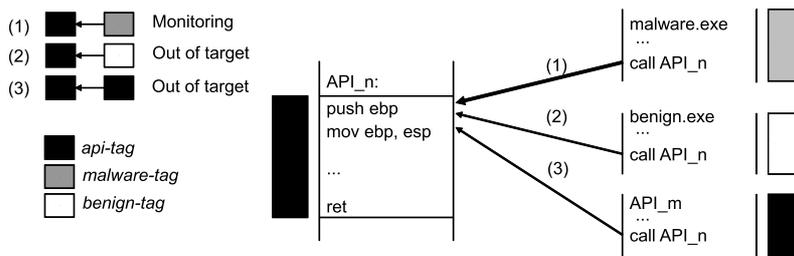
Fig. 2 Taint-based control transfer interception.
