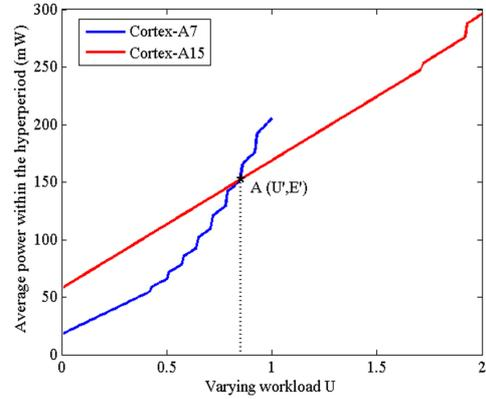
**Fig. 6** The energy relation of big and little cores with varying workload.
