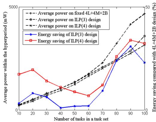
Fig. 8 A supplementary experiment on Big.Medium.Little architecture.
