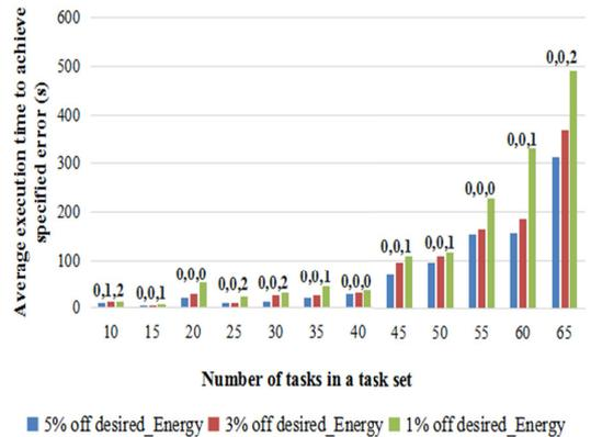
**Fig. 4** The effectiveness of Fast Terminate: average execution time to achieve specific percentage error.
