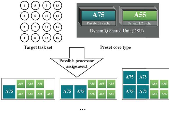
Fig. 1 Flexible core number design announced with DynamIQ technology.
