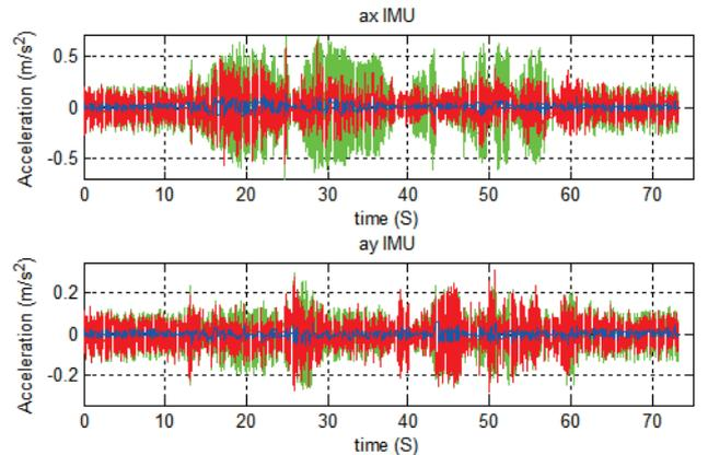
**Fig. 8** Acceleration on X and Y axes before filtering (green mark), after LMS filtering (red mark), and combined LMS and FIR filtering (blue mark) at random RPM.
