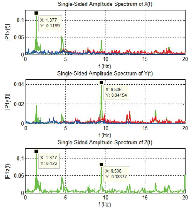
**Fig. 4** Spectrum in low frequency of IMU accelerometer axes before filtering (green mark), after LMS filtering (red mark), and combined LMS and FIR filtering (blue mark) at approximately 2,100 RPM.
