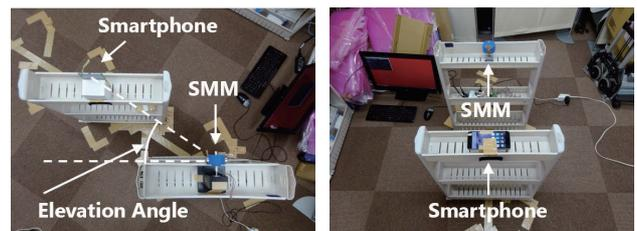
(a) Experiment for elevation angle  $\psi$  estimation (b) Experiment for azimuth angle  $\theta$  estimation
