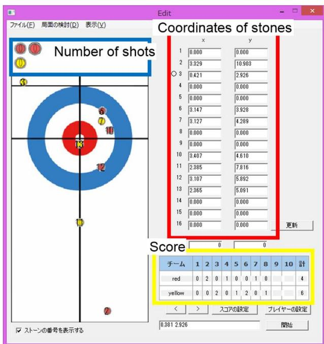
Figure 2: Interface of the game-state editor. Text boxes inside the red frame display the coordinates of stones. The blue frame shows the graphics of stones indicating the number of shots (or number of remaining stones). The yellow frame is the score board.
