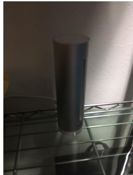
Fig. 4 Air temperature sensor in room
