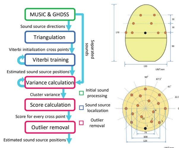
Fig. 1 On the left: Flow graph of the bird localization system, On the right: Egg-like shaped array design
