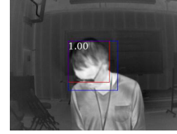
Fig. 4 The calibration network adjusts the detection window to be better aligned to the face region. The bounding-box (red) is generated from the face detector in the first stage, the bounding-box (blue) is the adjusted result.
