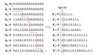
Fig. 3 Optimized probability array by deleting zeros at the right side of dotted line, the sign bit indicates the difference between two consecutive block lengths
