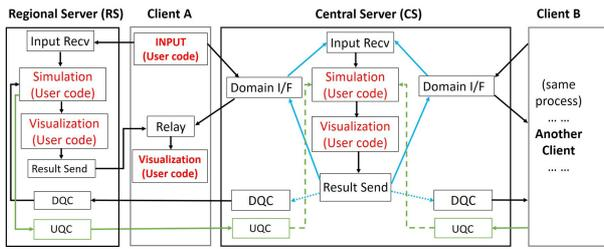
Fig. 2 The system design of Silk Road Framework.
