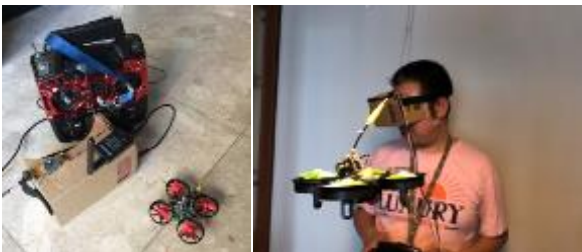
図 7 Cheap Flying Head の構成 Figure 7 Set of Cheap Flying Head.
