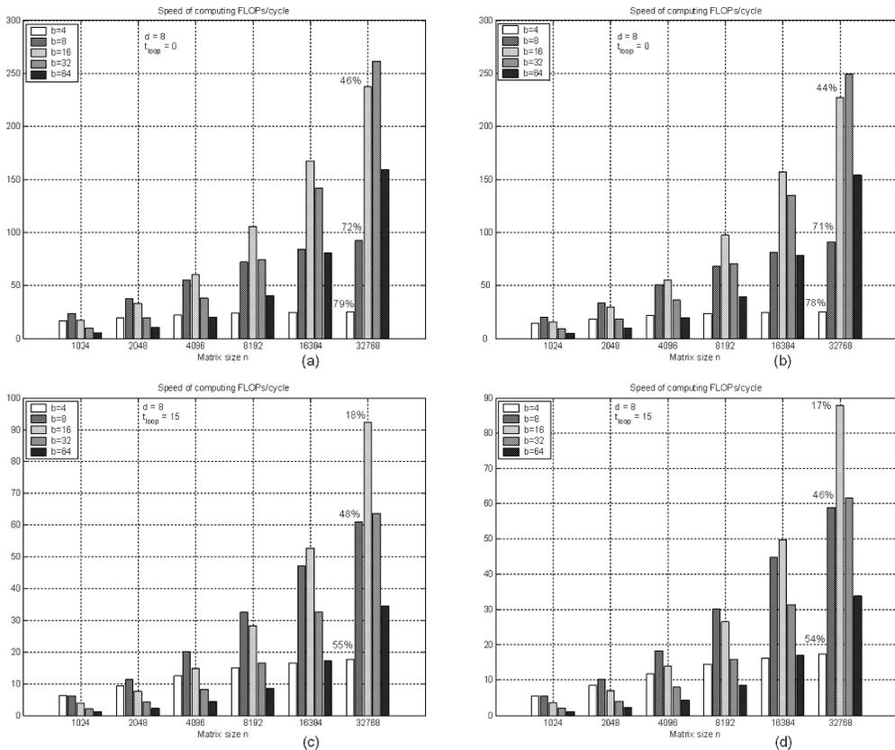
Fig. 6 Performance of the blocked LU factorization with  $d=8$ .
