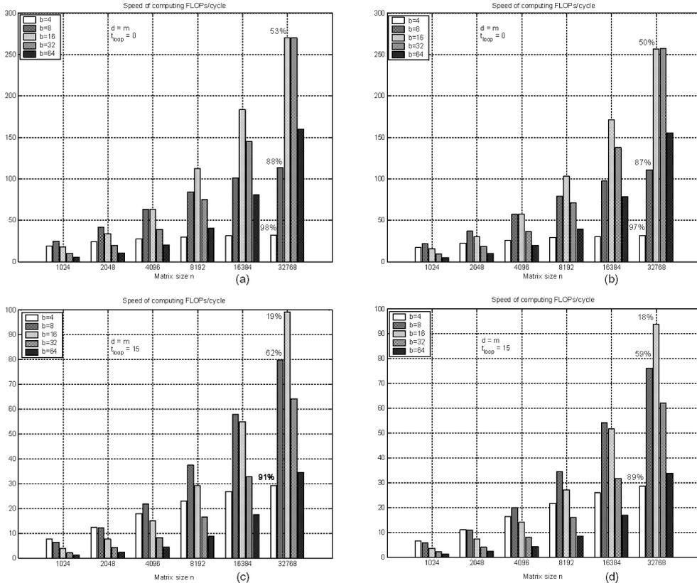
**Fig. 5** Performance of the blocked LU factorization with different matrix sizes and block sizes where  $d=m$ . The numbers on top of bars at  $n=32K$  are the percentages of the maximum speed attained.
