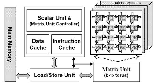
**Fig. 1** The proposed matrix processor block diagram.
