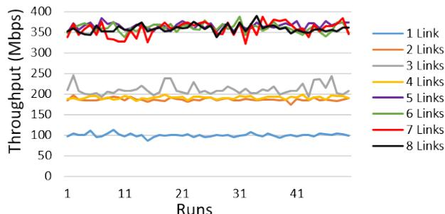
Figure 3: Throughput of each host (Link Aggregation)
