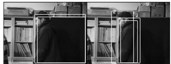
(a) another object with similar brightness (b) correction by target motion region
