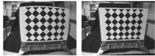
(a) Before distortion correction (b) After distortion correction
