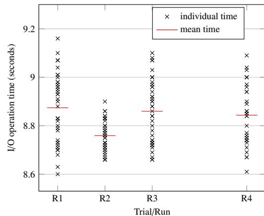
Fig. 7 IOR performance when writing to the on-node SSD on TSUBAME2.5 with placement B
