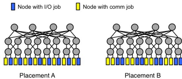
Fig. 2 The process-node mapping (node placement strategy) used in our experiments.
