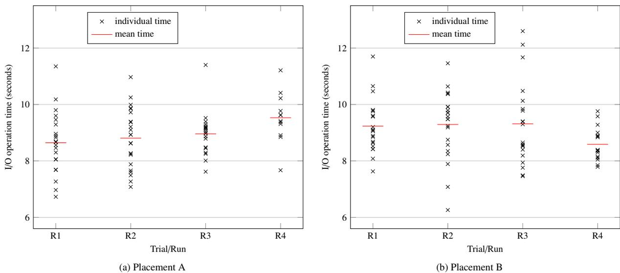
Fig. 5 IOR performance when reading from Lustre file system on TSUBAME2.5
