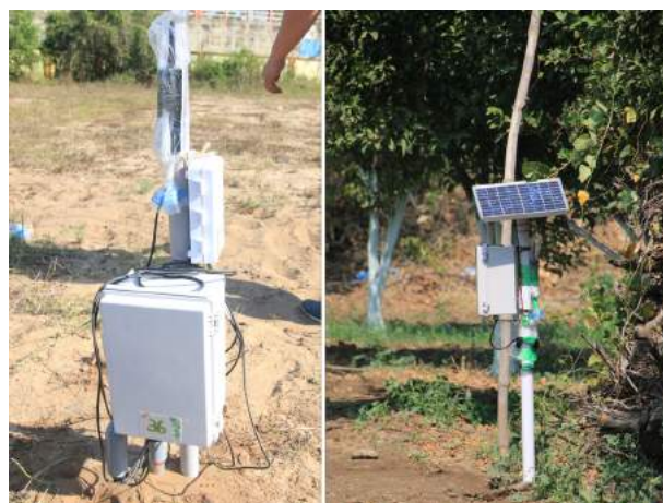
図 9 Deployment. Left: a slave node, Right: a master node
