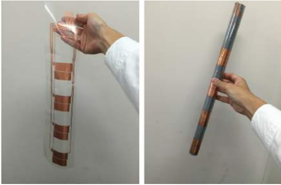
図 2 Left: soil moisture sensing pattern, Right: profile probe[15]
